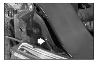
5. Remove the horizontal pin from the headlamp assembly by lifting the end of the pin upward until it unsnaps and then pulling it toward the center of the vehicle.
